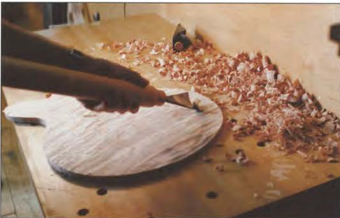
This page, top: Steve's exhibition table at the 2006 GAL Convention. Look closely to find Taku hiding behind the guitar. Above: Carving a maple back old-school with a whaling harpoon. I mean, a big fishtail gouge. Facing page, top: Using a violin-style depth marker punch. Bottom: A pivotal moment captured on black-and-white film. Steve has a front-row seat to see Guy Rabut demonstrate carving a violin scroll at the 1995 GAL Convention.
